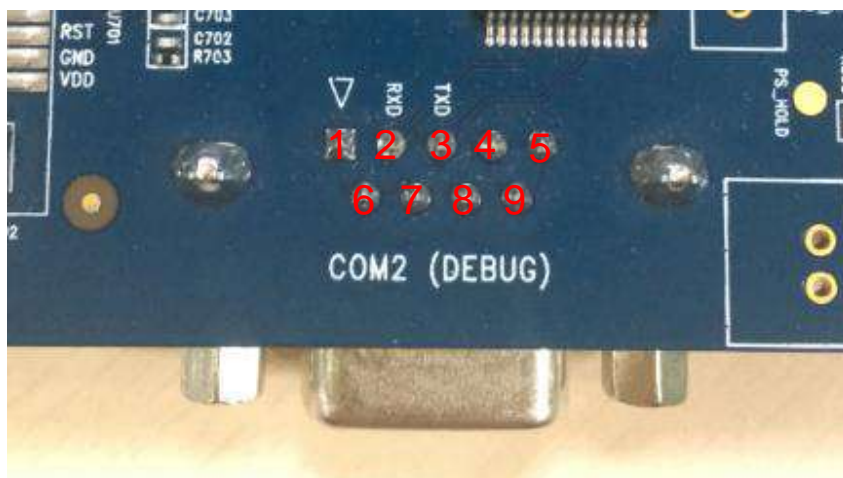
Figure 26: Pin Assignment of J402
