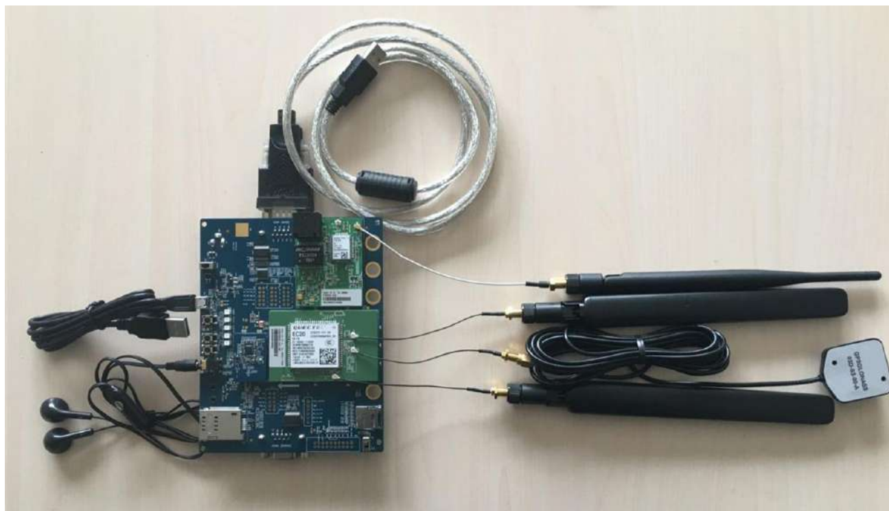
Figure 4: UMTS&LTE EVB Kit Assembly
