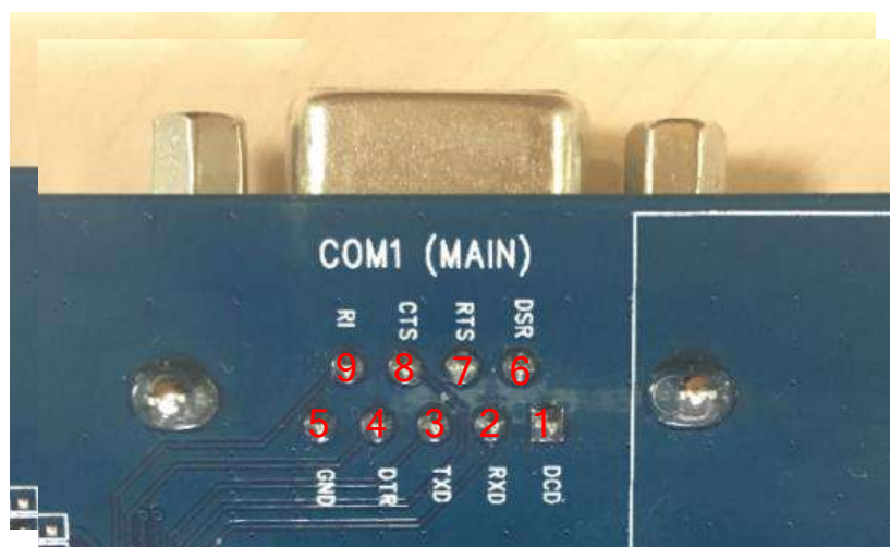
Figure 25: Pin Assignment of J401
